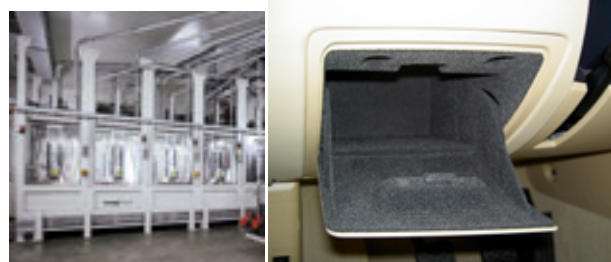
Flocking machine for gloveboxes / flocked glovebox
